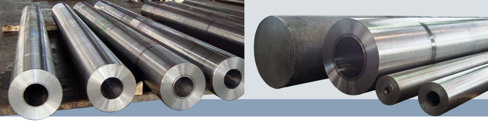
**Deep drilling**On items of every dimension starting from I.D. 30 mm and length up to 22 m.
