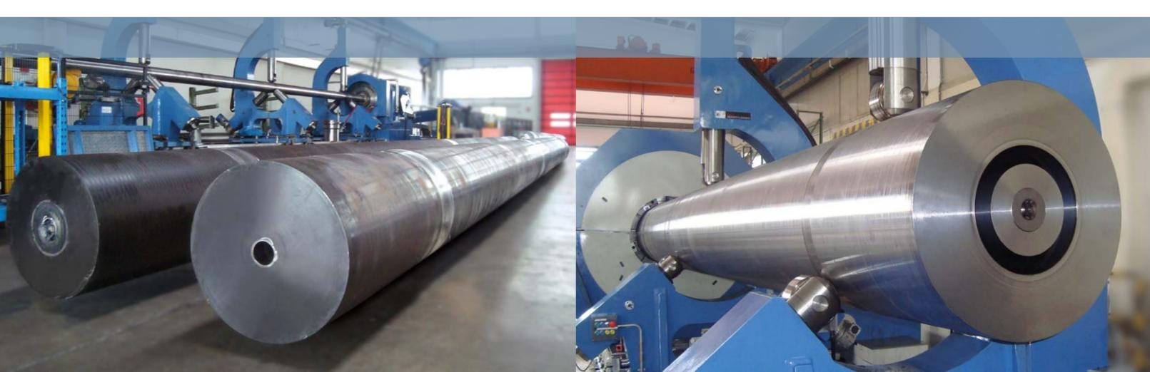
**Boring**Boring up to I.D. 1.200 mm and length up to 22 m in only one way.
